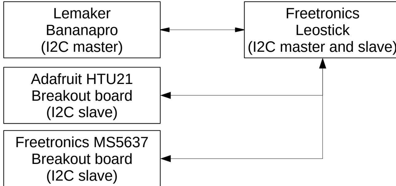
I was never completely satisfied with this setup but have used it for years not realising that the Linux kernel provided the **Industrial I/O subsystem** which allows for simple direct interface with **I2C** sensors.
