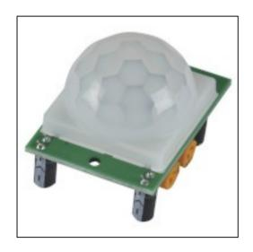
This sensor will run on 4.5-12VDC. Its logic voltage (output) is 3.3VDC out. This is compatible with the Raspberry Pi Zero's GPIO pins, i.e. 3.3VDC.
