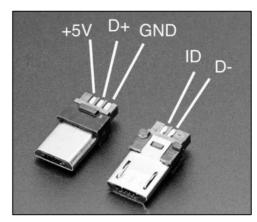
The C270 circuit board was removed from its enclosure and the usb cord was cut off leaving 200mm still attached. The cord was stripped leaving 4 wires which were soldered to an *Adafruit DIY Micro-B USB Plug*. Refer to the schematic for correct wire colours.
