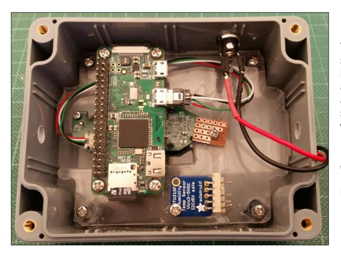
The perspex plate is secured to the enclosure bosses with 3mm screws and the Raspberry Pi Zero and HTU21 have been secured to their standoffs with 3 mm screws
