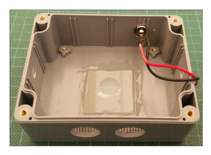
The remote webcam will be installed outdoors. In order to prevent insects taking up residence a piece of 1mm picture frame glass is placed over the webcam viewport and flywire is placed over the ventilation holes. Both are fixed in place with 2 part epoxy.
