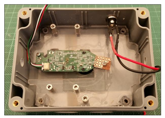
The webcam circuit board is fixed onto a piece of perspex over an opening large enough to allow for ventilation. A screw was used through an existing hole on one end. The other end was clamped in place with a piece of vero board.
