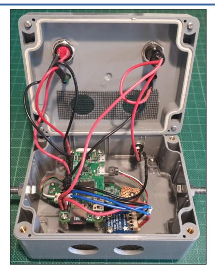
Left to right on the inside of the enclosure cover: the momentary pushbutton shutdown switch with green 5mm LED mounted in a black plastic bezel and the push button latching on/of switch with red LED in plastic bezel.
