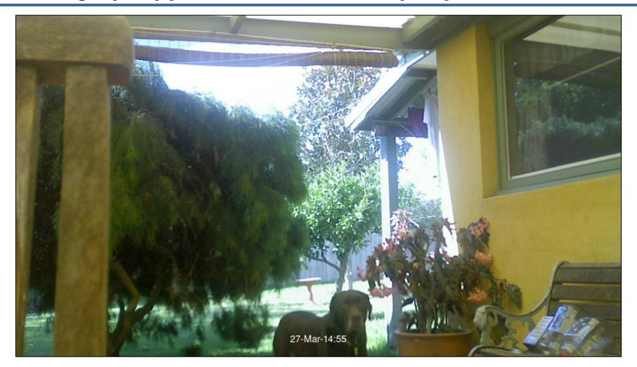
In the image on the previous slide our dog was ~3 metres from the sensor when it detected his movement. The acacia behind the dog was ~4 metres away from the sensor. The sensor detected the acacia branches moving in the breeze.
